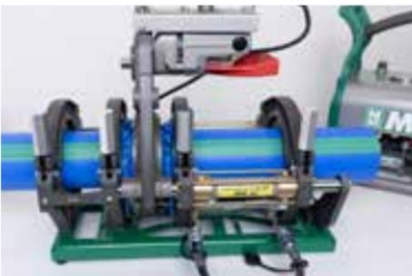
Start the facer and close the carriage starting with drag pressure, increasing pressure as necessary to produce ribbons of plastic from all 360° of both pipe faces.
