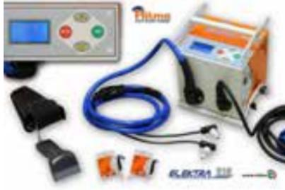
**Processor.** This device runs an electrical current at precise voltage and amperage for a prescribed amount of time through electrofusion fittings. Processors require copious amounts of electricity, the amount increasing parallel the diameter. Ritmo Elektra Series: Light, 500, & 1000; Widos ESI 2000.
