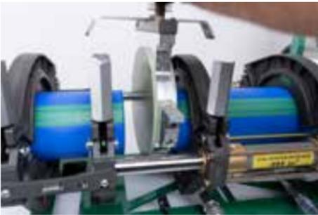
Upon completion of heating time, open the carriage just enough to successfully remove the heater plate and immediately close the carriage until the pipe faces touch and the machine is again at full pressure.
