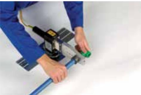
Once the material is fully loaded onto the adapters, begin the heating time countdown. As the heating time comes to an end, the beads on the components should begin to look shiny, almost appearing wet.
