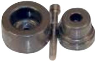
**Adapters.** An adapter is a set of machined aluminum, Teflon-coated bushings and will be necessary for each diameter of pipe to be socket fused. It is fastened to a heating iron and transmits heat from the iron to the PPR. POLOPLAST pipe and fittings are manufactured for adapters cut to the DVS Type A standard.
