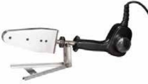
**Hand iron.** A hand iron is a heating element with a handle that comes in multiple sizes and is a core utensil on any socket fusion job. It is used for both hand-held and jig-assisted fusion. Examples: light small diameter bench mounted fabrication, in-line small-diameter fusion in tight places.
